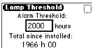
Figure 4–12: Lamp alarm threshold screen
