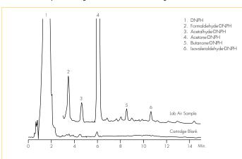
The above sample was collected in a chemical research laboratory using a portable sampling pump. One hundred liters of air was drawn through the cartridge at 0.65 L/min. The chromatogram shows ormaldehyde (4.8 ppbv), acetaldehyde (1.2 ppbv), acetone (118 ppbv), butanone (0.8 ppbv), and isovaleraldehyde (0.7 ppbv).
