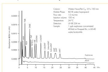
Achieve the lowest method detection limits using Waters Porapak RDX cartridges. The chromatogram above shows the analysis of reagent  $H_2O$  spiked at the 1 ppb level. The bottom chromatogram is a reagent  $(H_2O)$  blank.
