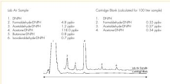
The sample was obtained in a chemical research laboratory using a portable sampling pump. One hundred liters of air was drawn through the cartridge at 0.65 L/min. The sample was found to contain low concentration of formaldehyde (4.8 ppbv), acetaldehyde (1.2 ppbv) and methyl ethyl ketone (0.8 ppbv), but a significant amount of acetone (118 ppbv). Significant concentrations of acetone are frequently found in laboratories because of its widespread use as a solvent.
