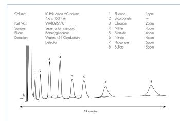
IC-Pak Anion HC (high capacity) columns use the same packing material as the IC-Pak Anion columns and are best suited for applications where there are orders of magnitude differences in the concentrations of the analytes. This is often the case with water and soil samples where you may have to measure ppb levels of phosphate in the presence of ppm levels of chloride and nitrate. The IC-Pak Anion HC column gives excellent resolution, even with injection volumes up to  $500~\mu L$
