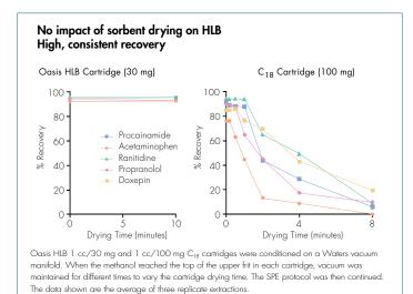
The variable recoveries seen with the  $C_{18}$  sorbents, due to the drying out effect, are often the cause for "retests", reducing laboratory productivity. In some laboratories 10% of samples are retests—this can be reduced using Oasis sorbents.
