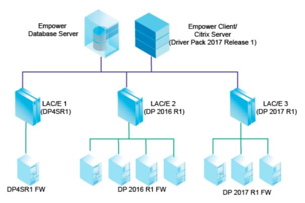
Alliance or ACQUITY instruments must have the firmware versions that are deployed with the driver pack installed on the Empower LAC/E.
