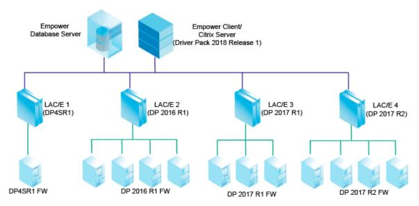
ACQUITY instruments must have the firmware versions deployed with the driver pack installed on the Empower LAC/E.
