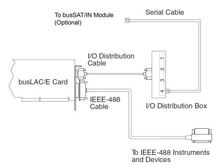
Triggering of devices, such as 2487, 2414, and 2410 detectors, occurs over the IEEE-488 cable and so requires no external trigger cables.
