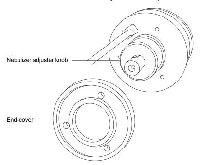
4. Unscrew and remove the nebulizer adjuster knob.
