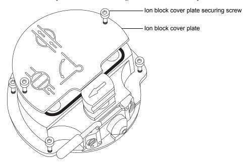
4. Remove the ion block cover plate.
