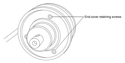
3. Remove the end-cover from the probe assembly.
