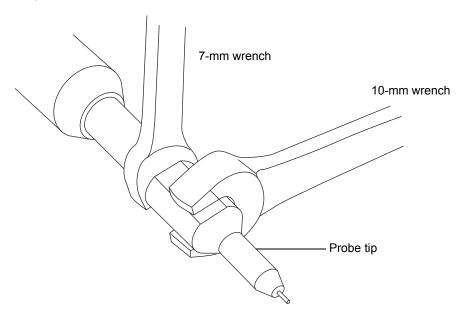
6. Remove the metal gasket from the probe tip.
