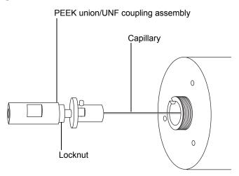
6. Use the 7-mm wrench to loosen the locknut.
