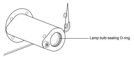
17. Use the O-ring removal kit to carefully remove the two O-rings from inside the lamp mounting flange (see "Removing O-rings and seals" on page 97).
