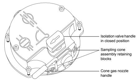
3. Grasp the cone gas nozzle handle and use it to rotate the sampling cone assembly through 90 degrees.
