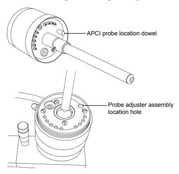
3. Tighten the probe locking ring to secure the probe in place.
