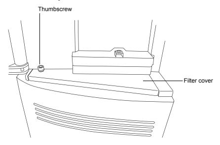
3. Remove the filter cover from the instrument.
