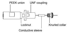
9. Remove the knurled collar and conductive sleeve from the capillary.
