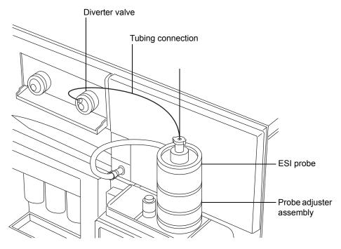
**Tip:** The other plumbing connections are omitted for clarity.
