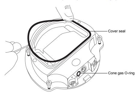
14. Use the O-ring removal kit to carefully remove the cone gas O-ring from the ion block.
