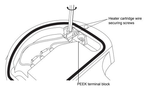
6. Use the needle-nose pliers to carefully swing the ring terminal tags out of the terminal block.
