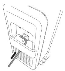
5. Insert the length of 4-mm nylon tube through the back of the lamp drive assembly, and push the bulb forward.
