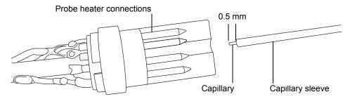
2. Carefully slide the probe heater over the capillary sleeve on the probe assembly.
