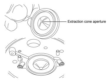
3. Remove the extraction cone handle insulator from the extraction cone handle.
