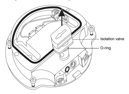
8. Use the O-ring removal kit to carefully remove the isolation valve O-ring (see "Removing O-rings and seals" on page 97).
