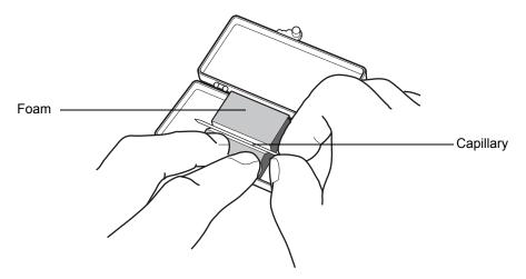
8. Load sample into the capillary using either a fused silica syringe needle or a GELoader<sup>®</sup> tip, minimizing any bubbles between the capillary tip and the sample.
