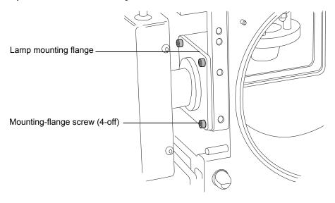
11. Slide the lamp assembly, shaft, and flange out of the APPI source enclosure.
