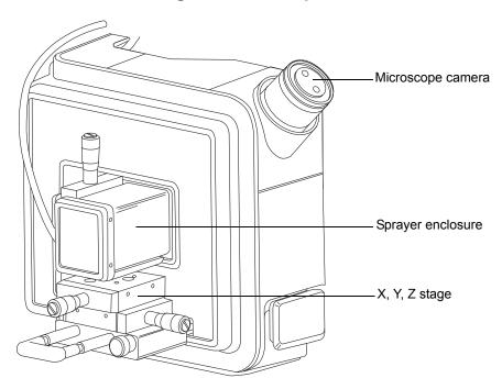
A sprayer is mounted on an X, Y, Z stage (three-axis manipulator) which slides on a pair of guide rails that allow its withdrawal from the source-enclosure for maintenance and changes.
