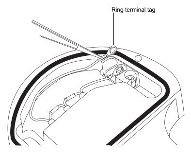
7. Use the needle-nose pliers to gently grasp the heat-shrink tubing on the heater cartridge assembly and slide the assembly out of the ion block.
