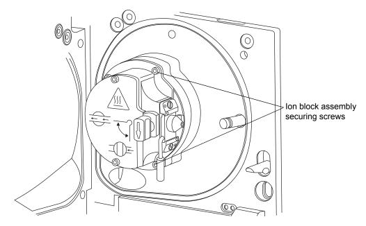
4. Remove the ion block assembly from the PEEK ion block support.
