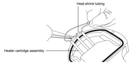
8. Dispose of the heater cartridge assembly.
