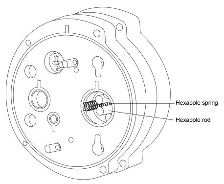
6. Fit the ion block assembly to the PEEK ion block support (see "Cleaning the source hexapole assembly" on page 140).
