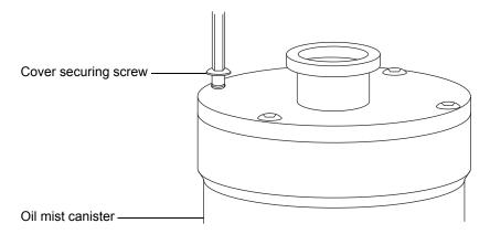
2. Remove the oil mist canister cover from the oil mist canister.
