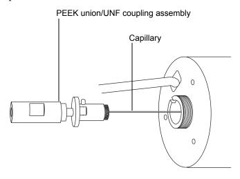
8. Unscrew and remove the knurled collar from the UNF coupling.
