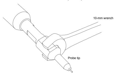
**Tip:** If the probe tip is difficult to remove, use the 7-mm wrench in conjunction with the 10-mm wrench.
