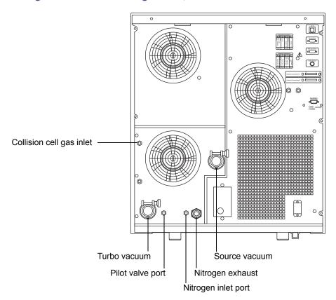
2. Attach a nitrogen regulator (not provided) to the nitrogen supply.
