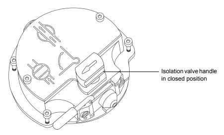
3. Use the combined 2.5-mm Allen wrench and cone extraction tool to loosen the 2 captive screws securing the ion block cover plate.
