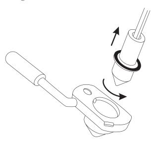
4. Remove the O-ring from the sample cone.
