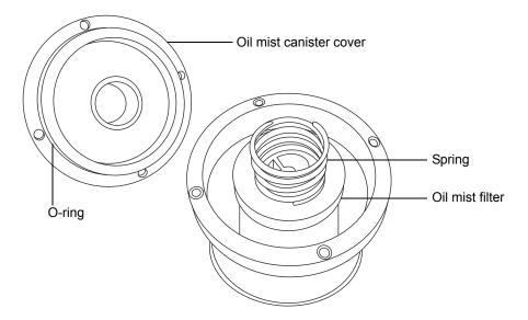
3. Remove the spring and oil mist filter from the canister.
