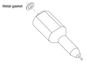
7. Remove the PEEK union/UNF coupling assembly and capillary from the probe.
