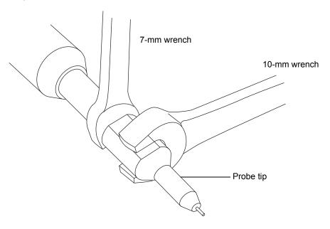
3. Remove the metal gasket from the probe tip.
