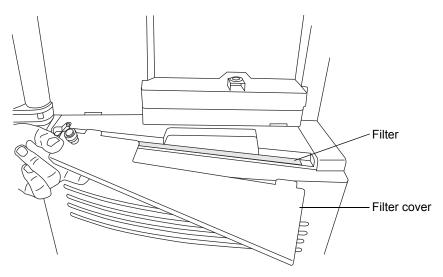
4. Lift the filter, vertically, from the its slot in the instrument.
