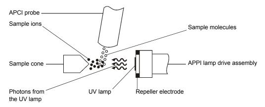
The APCI probe introduces vaporized sample into the source where photons generated by an ultra-violet (UV) lamp (mounted in the APPI lamp drive assembly) produce sample ions. Direct photoionization of a sample molecule occurs when the photon energy exceeds the ionization potential of the sample molecule.
