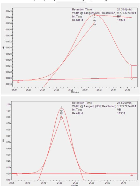
Peak Plot for the 2 adjacent peaks processed with original processing method and then manually integrated:
