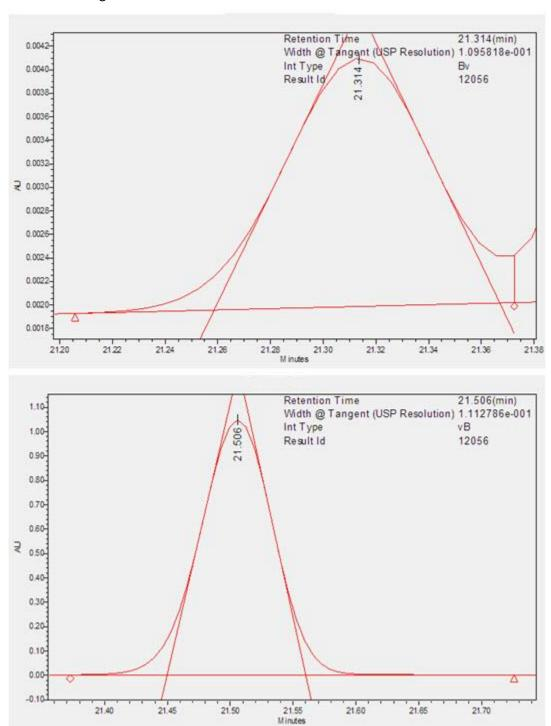
Peak Plot for the 2 adjacent peaks processed using E3 FR4 with original processing method except no Peak Width or Threshold settings (no default values nor integration events):
